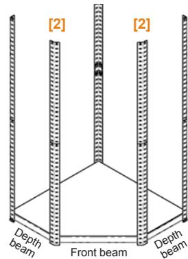
**STEP 5:** Join the two obtuse-angled front uprights [2] together by adding a front beam [8]
