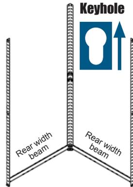
To add a width beam, strike its lugs firmly down into the "keyholes" of the uprights using a rubber mallet. Force is required. **NOTE: the lugs do not need to go completely to the bottom of the keyholes.** Pinch the beam and upright together using thumb and forefinger directly between the lugs to ensure they are located before hammering.
