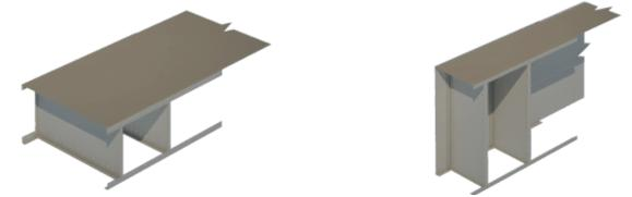
Finally add the base plate and ensure that its nuts and bolts are tightened securely.
