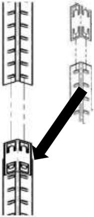
Fig1. (left) Splice 2 x uprights with 1 x splicing connector
